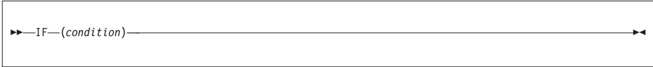
Option A tests the previously set condition code. It uses the Extended Branch Mnemonics for the branch instruction or the numeric condition code masks to indicate the condition. Table 3 following the examples shows the mnemonics and their complements.
